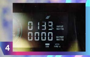
ONCE CONNECTED, THE SOLAR ICON WILL APPEAR IN THE BATTERY PACK DISPLAY.
