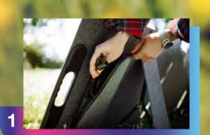
TAKE OUT THE WIRING HARNESS OF THE SOLAR PANEL.
