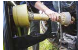
PTO drive shaft holder for easy and safety coupling
